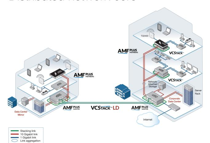
Today's corporate network users demand a high-performing enterprise network that can seamlessly carry multiple converged services, and provide instant access to online resources and applications. This key solution uses the x950 Series and VCStack LD—ideal for a distributed business network core that provides high availability, increased capacity and ease of management.
